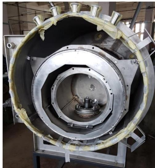
Fig. 7. Thermal conductivity measuring facility actual development
